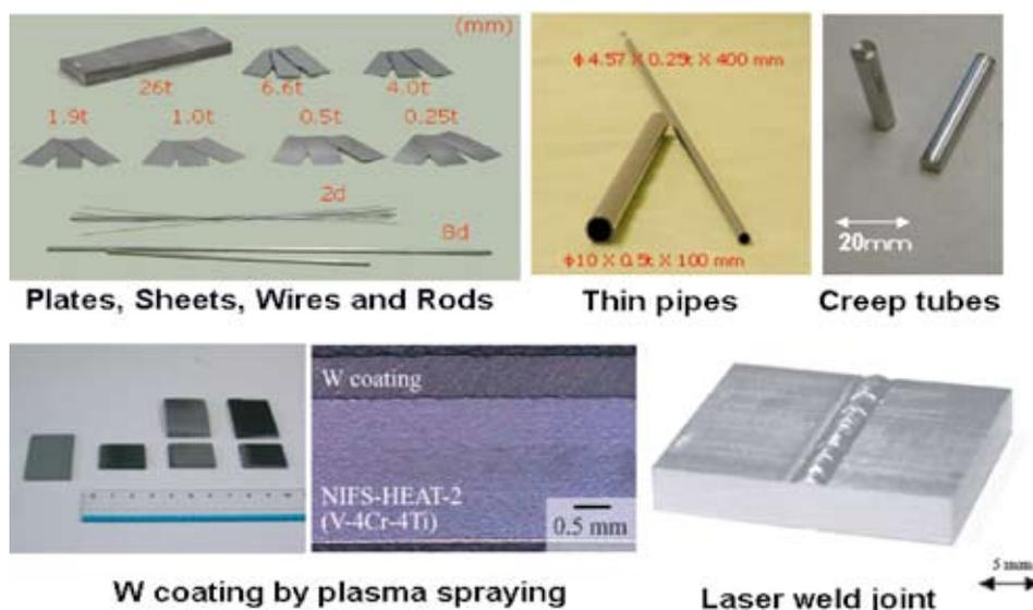
Fig. 1 Collection of the products of high purity V-4Cr-4Ti alloy.
