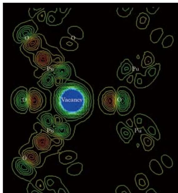
Fig. 2 Differential charge densities near oxygen vacancy
